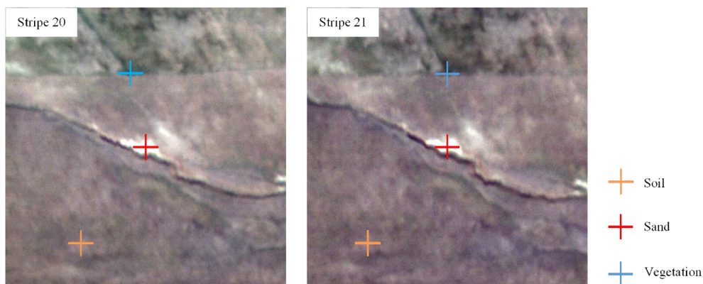
Fig. 11. The corresponding image points of adjacent strips acquired by HeadWall VNIR sensor.
