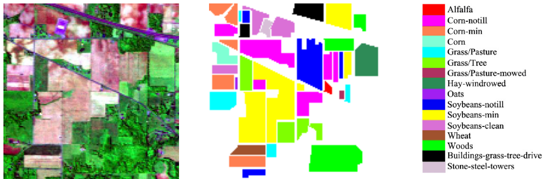
Fig. 6. Pseudocolor composite image and the corresponding ground truth for the Indian Pines AVIRIS data set.
