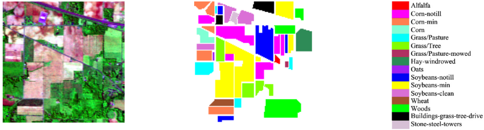
Fig. 8. Pseudo-color composite image and the corresponding ground truth for the Indian Pines AVIRIS dataset.
